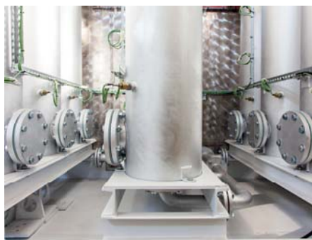
The back section of the REOIL unit where regeneration columns house sorbent, which ensures that all properties of the oil are sufficiently restored.
