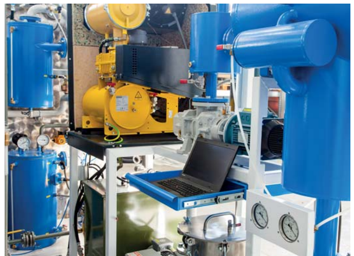
Fully automatic operation of the REOIL units is controlled by PLC while the operation is ensured by a SCADA system installed on a laptop.
